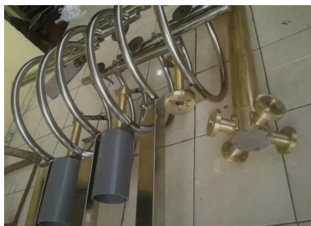
Figure 2. Omnidirectional antenna for FM TX
