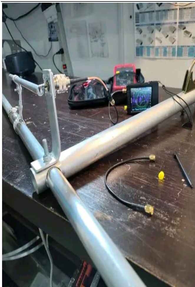
Fig. 2. Initial arrangement of the dipole radiating elements and supporting structure. Source: Authors' field photograph.
