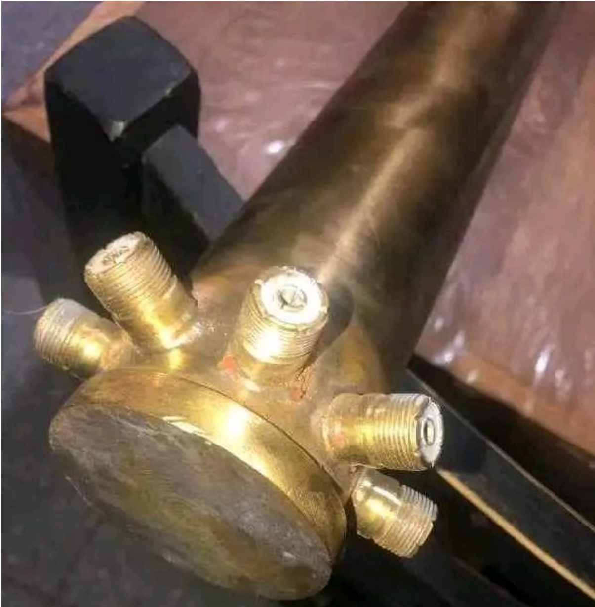
Figure 4: Antenna Combiner/Splitter coupling coil structure
