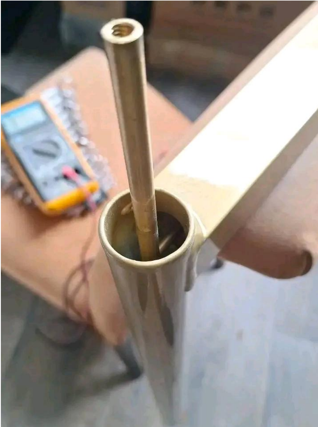
Figure 3: Antenna Inductive Coupling and Adjustment Mechanism for MICE Resonant System
