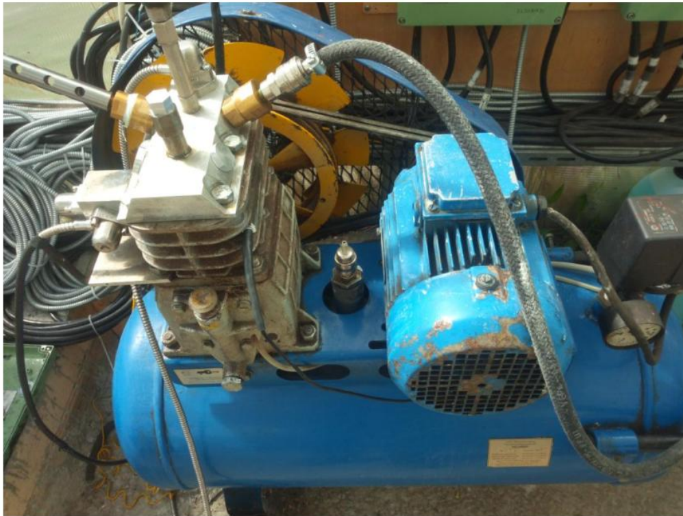
Figure 1: The compressor. The signal used for the fault detection monitoring was acquired from vibration acceleration probe mounted on the top of the cylinder.
